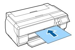
While aligning the right edge of the paper with the guide on the right-hand side of the tray, slide the paper all the way into the printer, and pull back the paper until the leading edge touches the tray.
