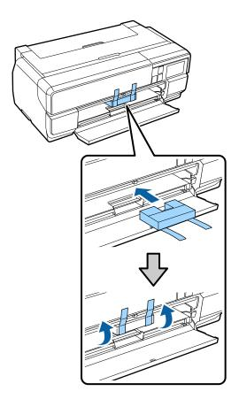
Close the front cover and secure it with commercially available tape and so on.
