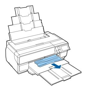
Open the printer cover and slowly pull the jammed paper out of the printer.
