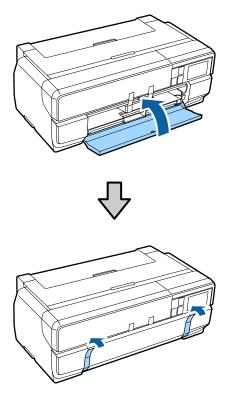
6 Keeping the printer flat, pack it in Styrofoam or other protective material and place it in the box.
