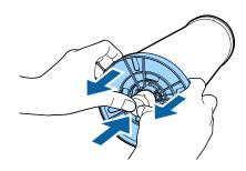
If it is difficult to remove, tap gently on the tip of the spindle on the black flange side.
