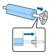
Press the black flange so that there is no gap between the flange and the roll paper.
