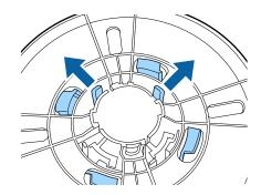
In the same way, push out the hooks and remove the attachment from the flange that is fixed to the spindle.
