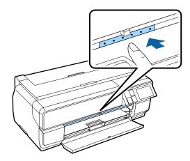
Load the paper vertically with the printable side face up.
