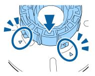
In the same way, insert the attachment into the spindle first, and then attach it to the flange that is fixed to the spindle.
