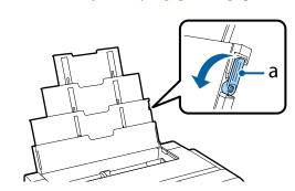
Pinch the edge guide and slide it to fit to the width of the paper.
