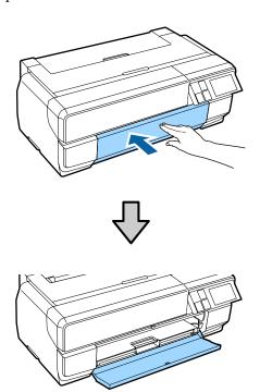
If you have changed the angle of the control panel, press and return it to its original position.
