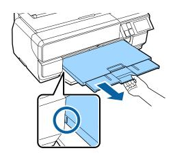
Load the paper vertically with the printable side face up.
