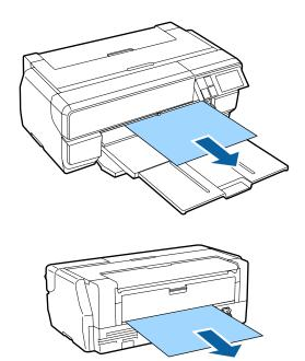
Open the printer cover and slowly pull the jammed paper out of the printer.
