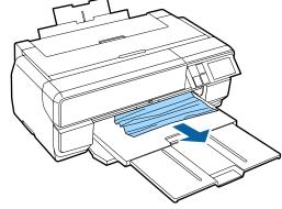
Open the printer cover and slowly pull the jammed paper out of the printer.
