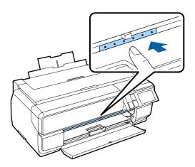
6 Load the paper vertically with the printable side face up.
