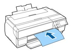
While aligning the right edge of the paper with the guide on the right-hand side of the tray, slide the paper all the way into the printer, and pull back the paper until the leading edge touches the tray.
